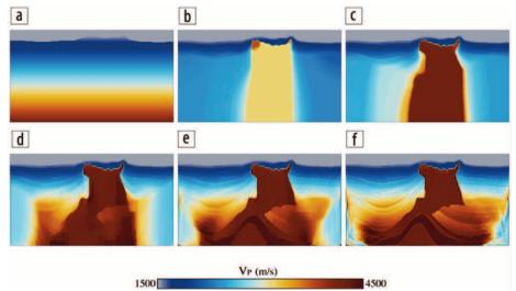
**Figure 6.** Evolution of the SEAM model from the starting point to the final recovered model as the constraints are relaxed. An accompanying video (viewable at http://library.seg.org/doi/suppl/10.1190/tle35030235.1) shows the full sequence of models.
