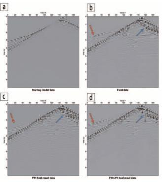
**Figure 5.** Shot records for (a) the starting model, (b) the true model, (c) final conventional unconstrained FWI result, and (d) the final hinge-loss constrained FWI result. Red and blue arrows highlight the parts of the data that are not properly matched with FWI without hinge-loss constraints.
