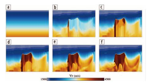
**Figure 3.** Snapshots for (a) the starting, and (b–f) the recovered velocity models, with one-sided TV continuation where the value of  $\xi/\xi_{true}$  is equal to (b) 0.01, (c) 0.1, (d) 0.2, (e) 0.5, and (f) 0.9. Adapted from Esser et al. (2015).
